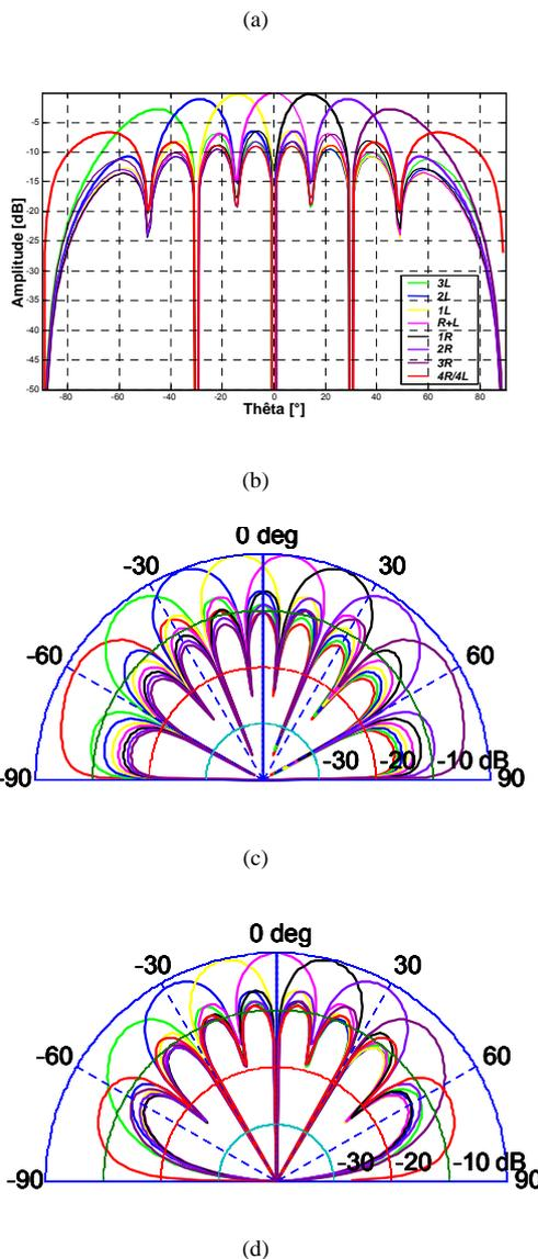
Fig. 5 Performance of the Butler matrix 8x8 standard (a),(b): Simulated radiation pattern in Cartesian coordinates respectively 3 dB/ $90^\circ$  couplers and 3 dB/ $180^\circ$  couplers (c),(d) : Simulated radiation pattern in polar coordinates 3 dB/ $90^\circ$  couplers and 3 dB/ $180^\circ$
