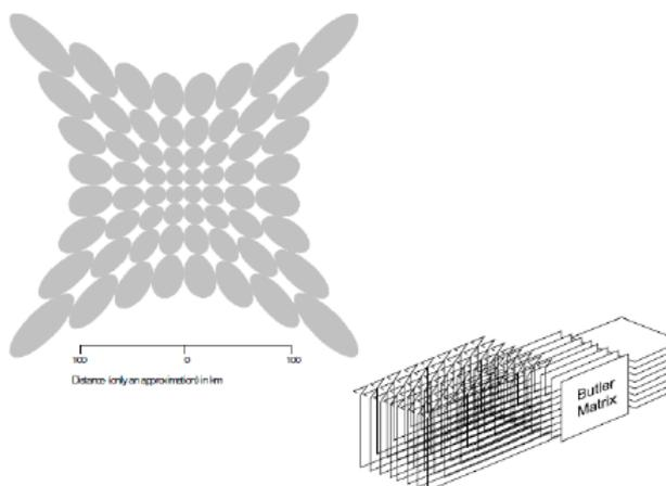
Fig .6 A two-dimensional Butler matrix producing orthogonal beams[7]
