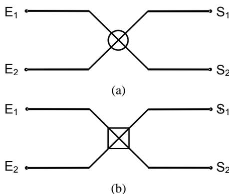
Fig. 1 Functional representation (a) 3 dB coupler 90°, (b) 180° 3dB couplers.
