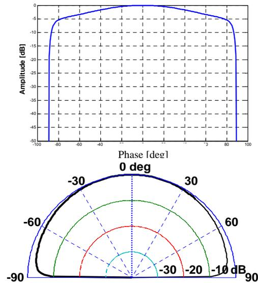
Fig. 3 Radiation pattern of a printed antenna at 10 GHz (a): Radiation pattern of a printed antenna (b): in polar coordinates
