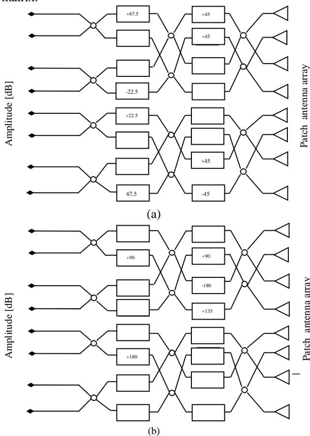
Fig. 4 Functional schematic Butler matrix (a):with 3 dB/ $90^\circ$  couplers (b) :with 3 dB/ $180^\circ$  couplers
