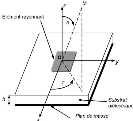
Fig. 2 Microstrip patch antenna
