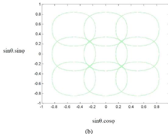
Fig. 7 Performance of the Butler matrix plan 4x4 standard (a): Three-dimensional radiation pattern (b) Two dimensional amplitude distribution on the aperture
