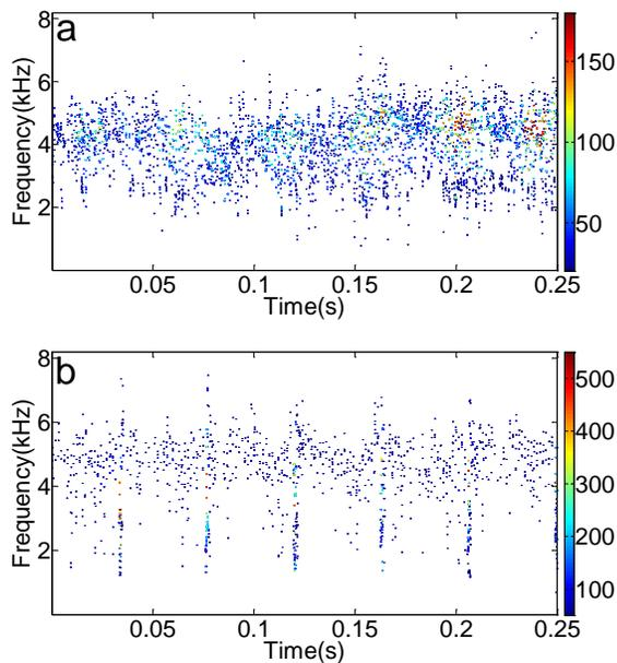
Fig. 6 The HHT spectra of the two vibration signals using the EEMD method: (a) The normal gearbox signal; (b) The broken-tooth gearbox signal.
