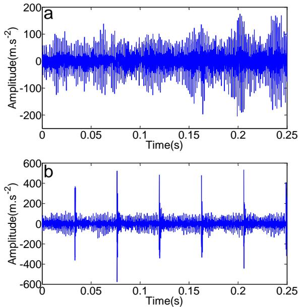
Fig. 5 The two gearbox vibration signals: (a) The normal gearbox signal; (b) The broken-tooth gearbox signal.
