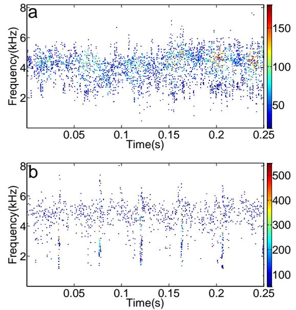
Fig. 7 The HHT spectra of the two vibration signals using the CEEMD method: (a) The normal gearbox signal; (b) The broken-tooth gearbox signal.
