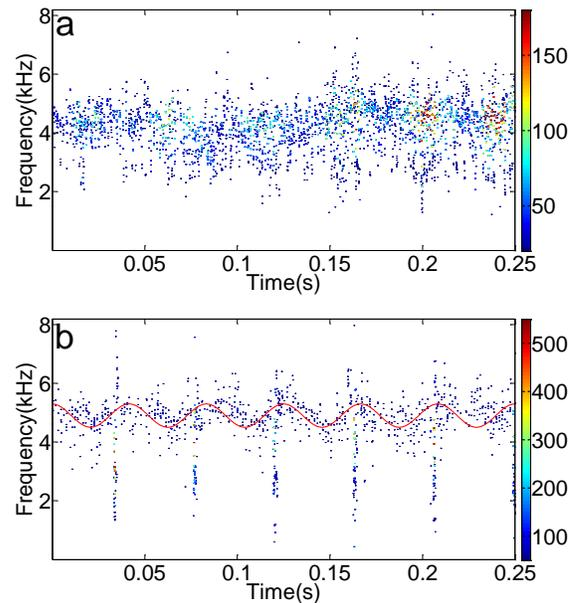
Fig. 8 The HHT spectra of the two vibration signals using the ICEEMD method (The red cosine curve is added to highlight the instantaneous frequency curve.): (a) The normal gearbox signal; (b) The broken-tooth gearbox signal.
