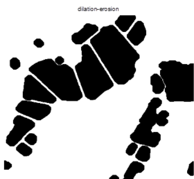
Fig. 10 Dilation followed by erosion using 2x2 structural elements
