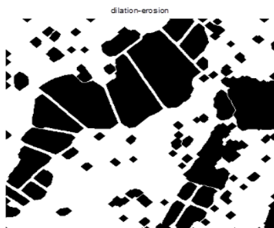
Fig. 10 Dilation followed by erosion using 2x2 structural elements
