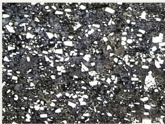
Fig. 6 Original image which represents the dispersion of TiB2 grains in the matrix of Iron.
