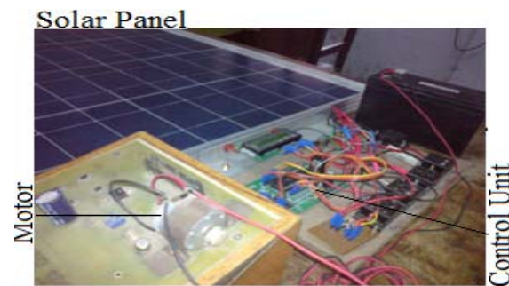
Fig.12. Snapshot of the Experimental setup showing the fabricated closed loop buck converter with MPPT algorithm and DC Motor for water pumping application.
