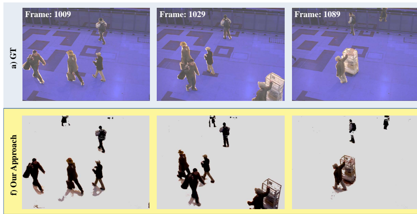
Figure. 6: shows the segmentation result from our segmentation algorithm in test sequence.
