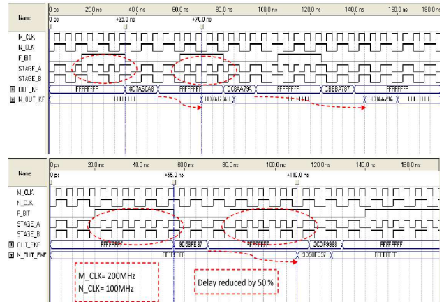
Fig. 3 KF and EKF output with\out flag-bit and flicker clock effects
