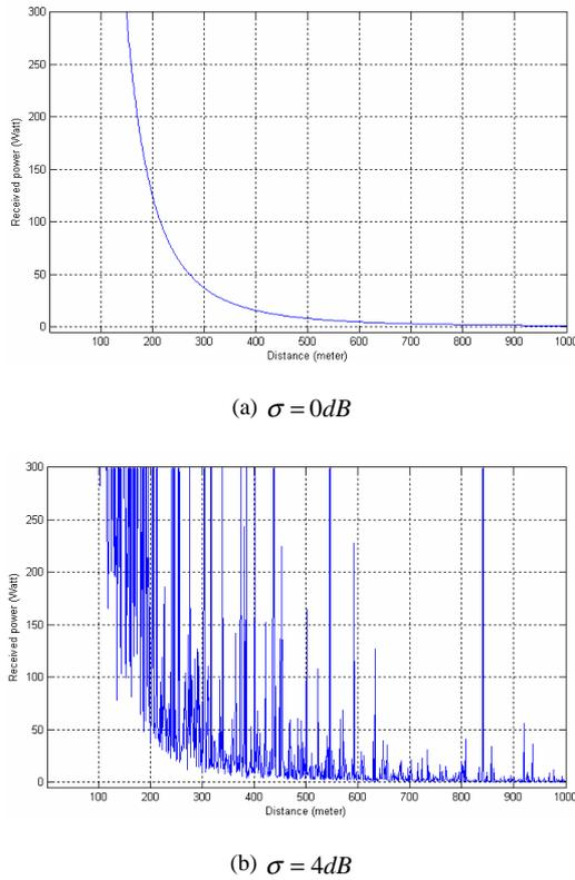
Fig. 1 The received signal power vs. the distance at (a)  $\sigma = 0dB$ , and (b)  $\sigma = 4dB$ .
