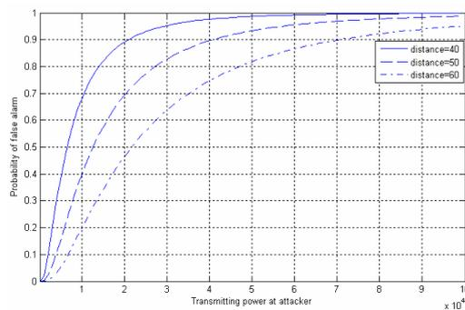
Fig. 5 Probability of false alarm vs. the transmitting power at the attacker for different distances
