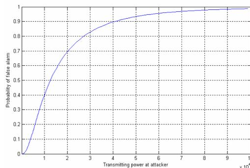
Fig. 4 The probability of false alarm vs. the transmitting power at the attacker at  $\gamma = 100$  watt
