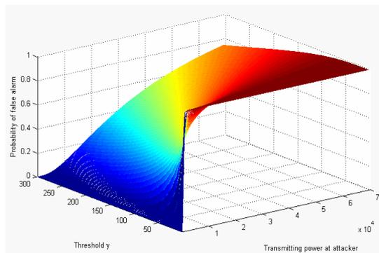
Fig. 3 The probability of false alarm and the threshold  $\gamma$  vs. the transmitting power at the attacker.
