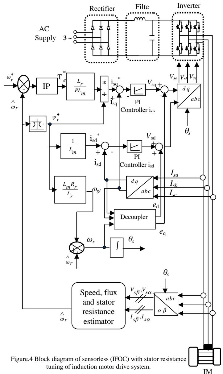
Figure.4 Block diagram of sensorless (IFOC) with stator resistance tuning of induction motor drive system.
