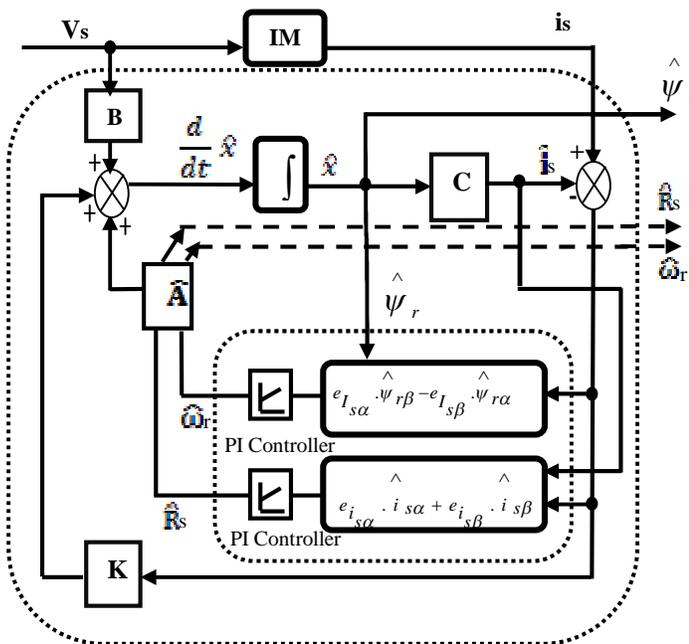
Figure 3. Block diagram of simultaneous estimation of rotor speed and stator resistance
