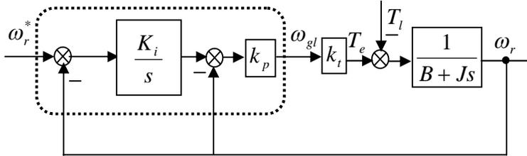
Fig.1 Bloc diagram of IP speed controller
