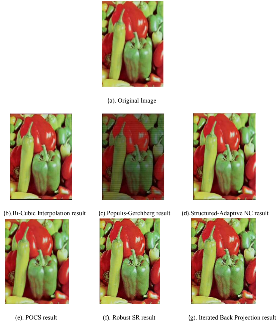
Figure 2: Comparison of Reconstruction Algorithms: (a) Original image (b) Bi-Cubic Interpolation results with HCI 0.0698 (c) Populis-Gerchberg results with HCI 0.4275 (d) Structured-Adaptive Normalized Convolution results with HCI 0.0653 (e) POCS results with HCI 0.0688 (f) Robust Super-Resolution results with HCI 0.1184 (g) Iterated Back Projection results with HCI 0.1343.
