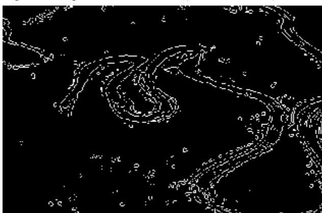
Fig. 4.6: Output of LoG Filter (Extracted Road)
