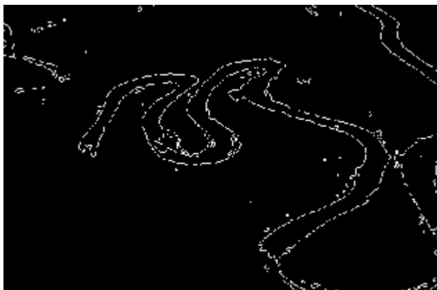
Fig. 4.5: Output of Prewitt Filter (Extracted Road)
