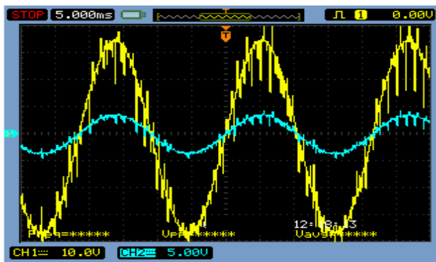
Fig.7 Input Voltage and Current waveform
