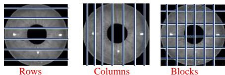
Fig. 4. Data partitioning techniques: horizontal (left), vertical (middle), block (right).
