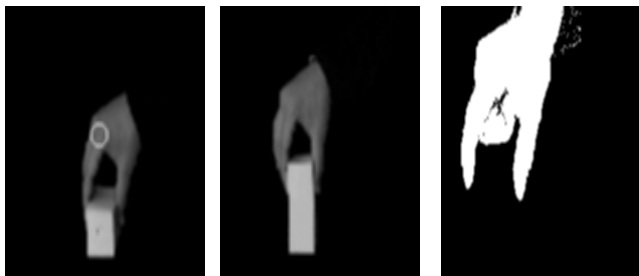
Fig. 2. In the left is the input image with a circle about the region that we try to find its correspondence in the second image, a segmented skin region according to Eq. (9), and Eq. (10) in the right respectively.
