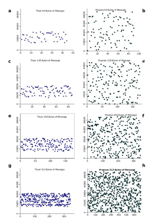
Fig. 3 The result of the DNS ID values based on 4 different messages sizes ranging from 64, 128,256 and 512 bytes. In the left side of the figure, labels a, c, e, and g are the result from the Tyher CC, while labels b, d, f, and h are the result of the DNS ID values from the proposed CC
