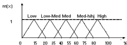
Fig. 4: Derived Triangular membership function
