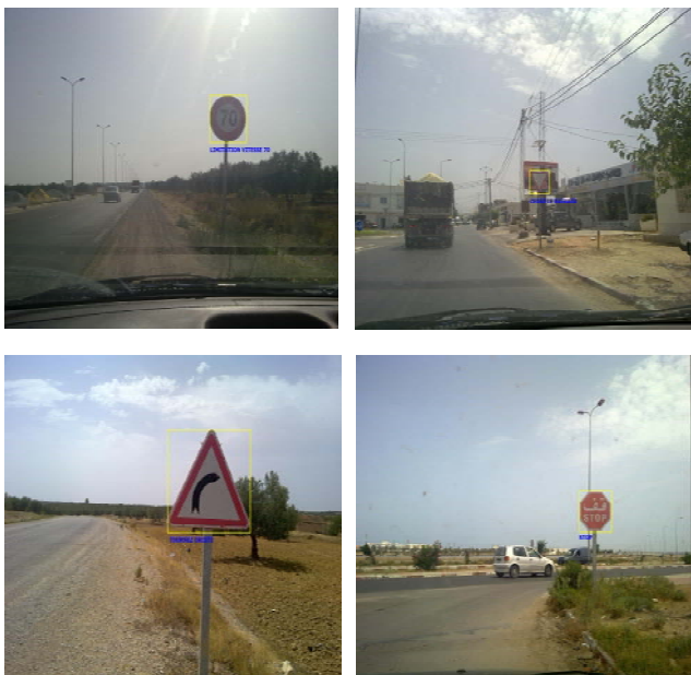
Fig. 10. Some results of the road sign recognition module
