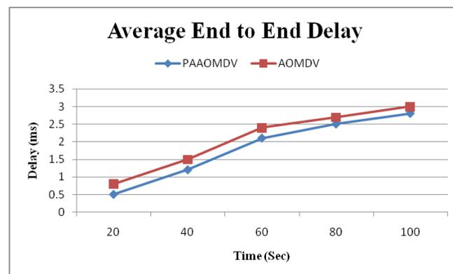
Fig. 2 End to End delay comparison.
