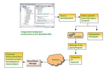
Fig.1 Working of ODRA (Object oriented database for Rapid application development)
