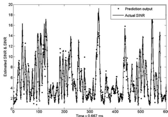
Fig. 15 The prediction output of SINR at the speed of 60 km/h along with the actual SINR.
