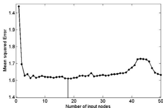
Fig. 13 MSE of different Adaline models at the speed of 120km/h
