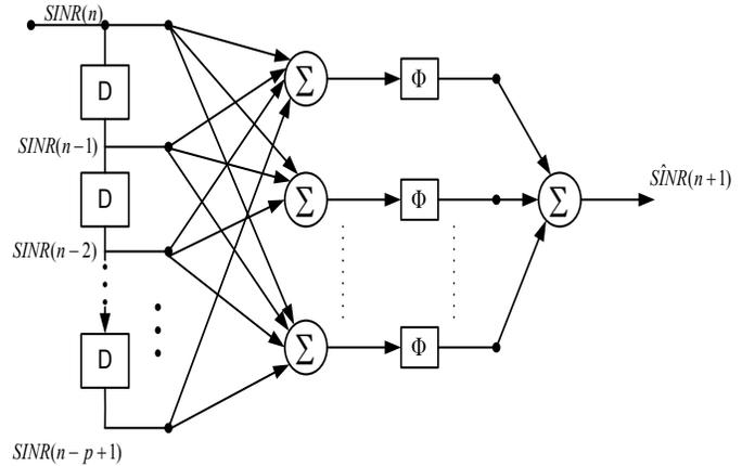
Fig.6 The structure of MLP neural network based predictor.
