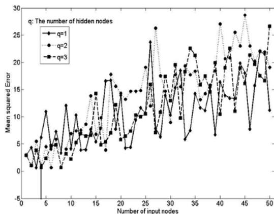
Fig.9. MSE of different MLP models at the speed of 60km/h.
