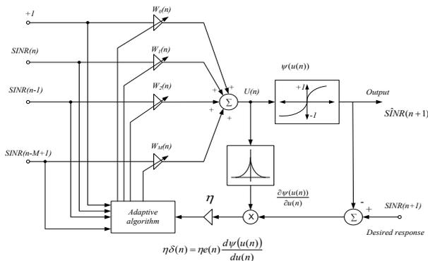
Fig.3 Diagram of back propagation learning algorithm
