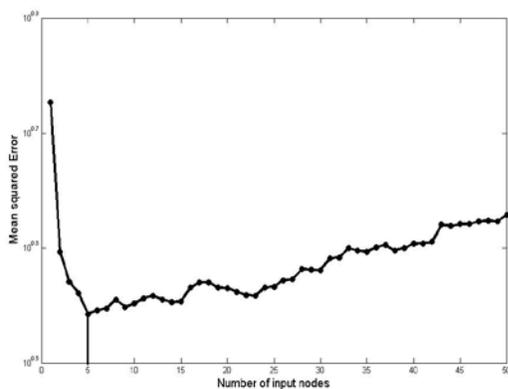
Fig. 12 MSE of different Adaline models at the speed of 60km/h
