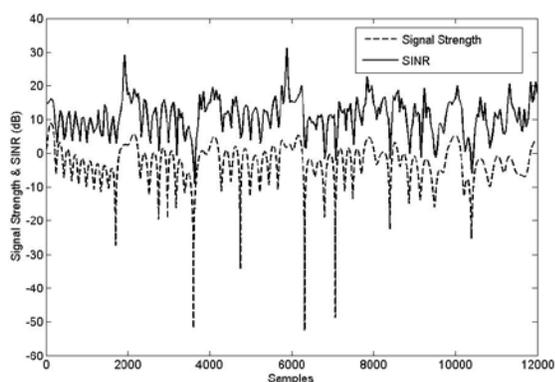
Fig.5 SINR in Rayleigh fading ( $f_D = 17Hz$ , with  $K=12$ )
