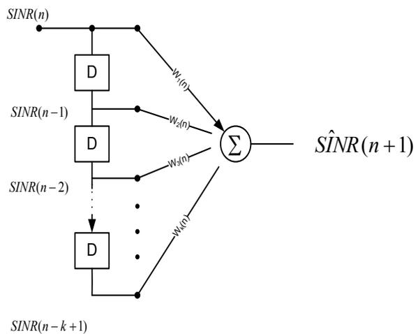
Fig.7 The structure of Adaline neural network based predictor
