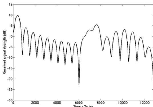
Fig.4.simulated Rayleigh fading ( $f_D = 50Hz, T_s = 15.625\mu s$ )
