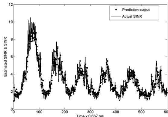
Fig. 14 The prediction output of SINR at the speed of 10 km/h along with the actual SINR.
