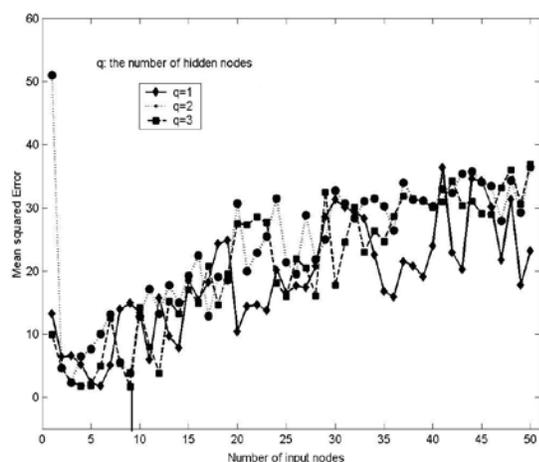
Fig.10 MSE of different MLP models at the speed of 120km/h
