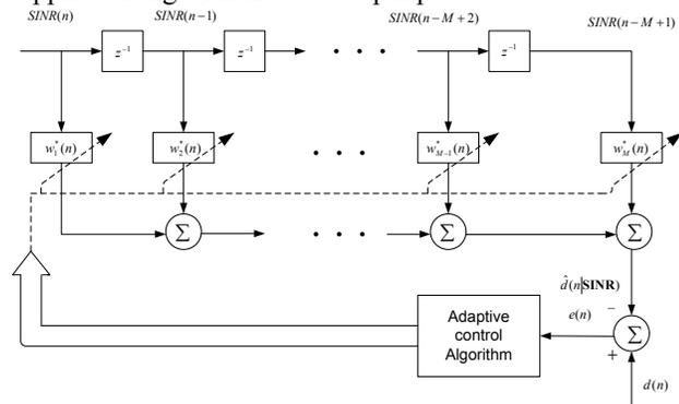
Fig. 2 Adaptive Filter in predictor application with SINR input
