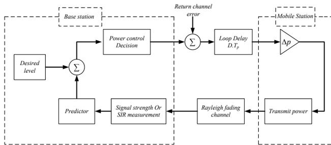
Fig.1 Closed-loop power control model
