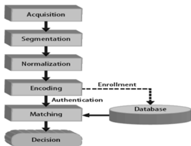
Fig 3. Frame work of iris recognition
