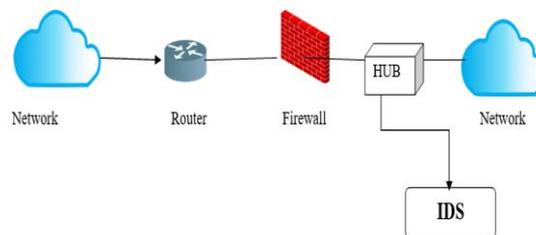
Figure 1.2: Position of IDS in an secure network
