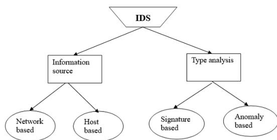
Fig 3. Intrusion Detection system types
