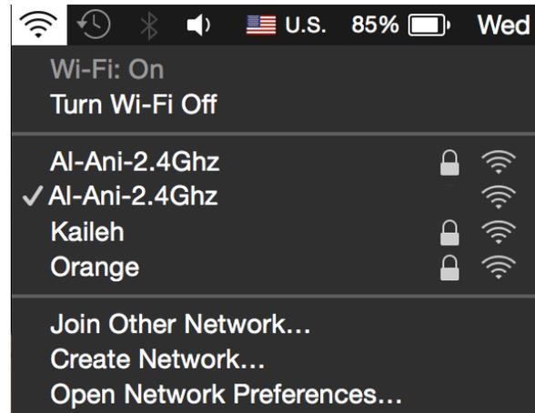
Fig. 3 The victim is now connected to the rogue access point
