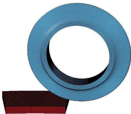
Fig. 2 3D finite element model of rock-breaking of a cutter
