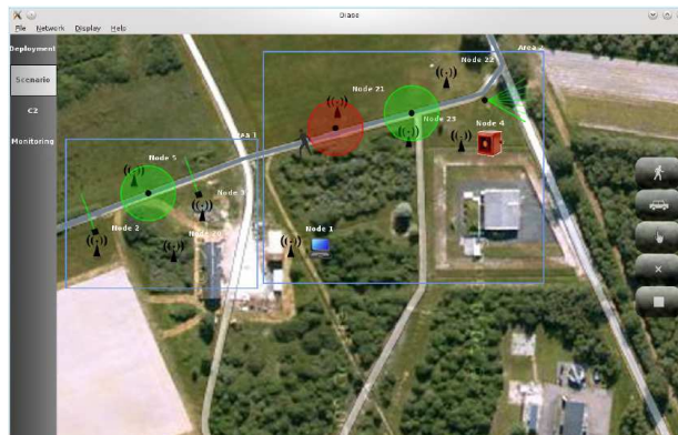
Figure 8: Screenshot of Diase running an intrusion scenario in real time and injecting simulated events to the emulated wireless nodes.
