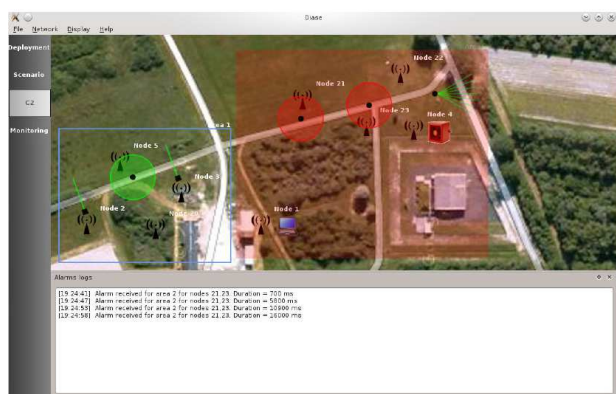
Figure 7: Command & Control mode: Visualization of an alarm in an area along with which sensors participated in it
