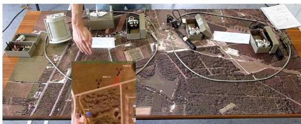
Figure 13: Testing the inter-area communication to decrease the intrusion detection latency
