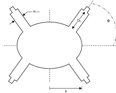
Fig. 4. Elliptical coupler using single layer.
