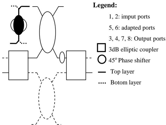
Fig. 1 Block diagram of multilayer six-port circuit based on Slot Coupled Directional Coupler.
