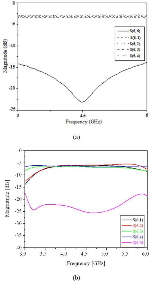
Fig. 7. Simulated S-parameters, (a). Simulation with CST. (b). with ADS.
