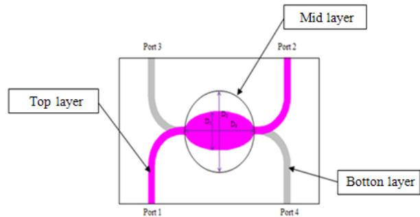
Fig. 2 Elliptical coupler using multi-layer technology.
