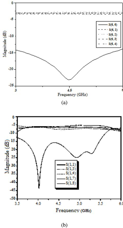
Fig. 9. Simulated S-parameters, (a). Proposed six-port junction. (b). conventional six-port junction.
