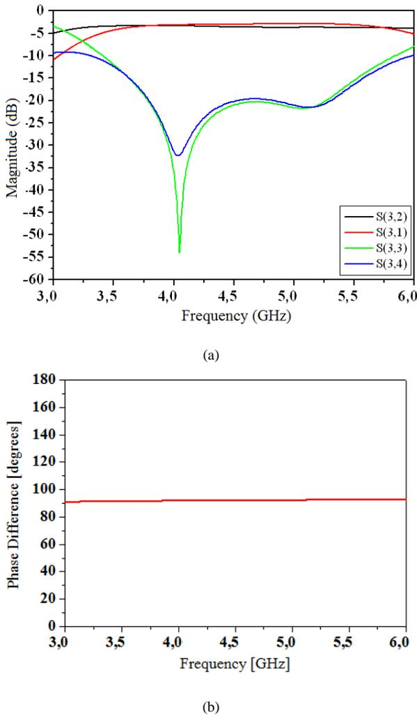
Fig. 5. Simulation results of S-parameter of elliptical coupler with ADS momentum. (a) Magnitude (b) Phase Difference.
