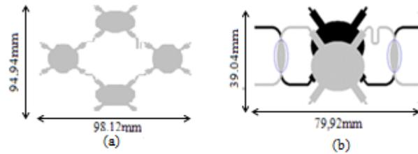
Fig. 6. (a). Layout of proposed six-port junction, (b). Layout of conventional six-port junction.
