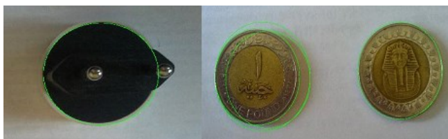
Fig. 6 Applying the CHT to three objects, the shades affect the detection of the coin in the middle.
