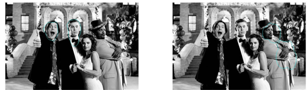
Figure 7. The top image represents the result of blobbing from the 2-person group while the bottom image represents the result of blobbing from the remaining group. Note that there is potential for error: some ellipses may persist through the safety nets and obscure itself as a "facial object".
