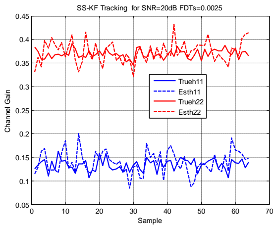
Fig.5 Tracking of channel coefficients h_{11} and h_{22} with SS-KF, for RSB = 20 \text{ dB} and f_D T_s = 0.0025 .
