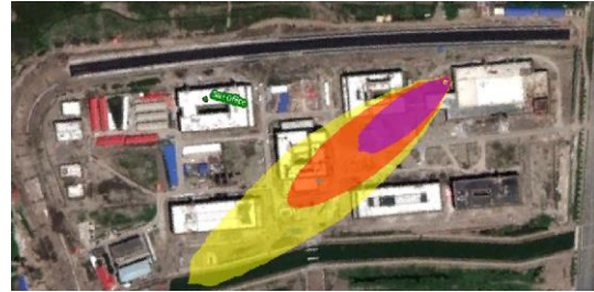
Fig. 6 Gas diffusion simulation based on WSN
