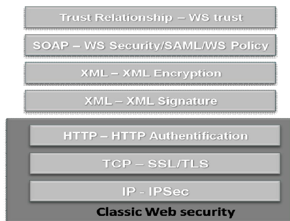
Figure 10: WS security stack
