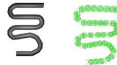
Fig. 2. Tubular objects are approximated with spheres [1].
