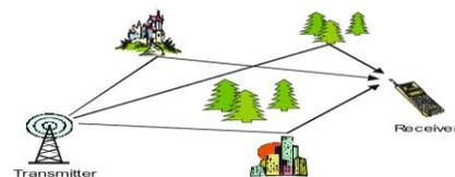
**Fig. 2 Multipath Propagation Scenario**
