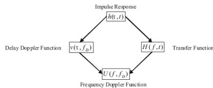
Fig. 5 Relationships between different system functions
