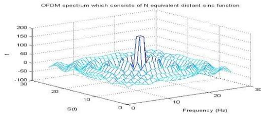
Fig. 7-b OFDM spectrum of N equidistant sinc functions simulated by Simulink
