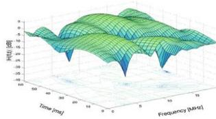
Fig. 4 Frequency-selective and time-variant radio channel transfer function
