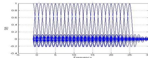
Fig. 7-a OFDM spectrum of N equidistant sinc functions simulated by Simulink
