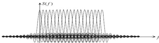
Fig. 6 OFDM spectrum which consists of  $N$  equidistant *sinc* functions
