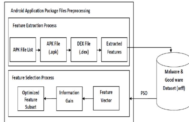
Fig. 4 The Developed SwarmDroid IDS Architecture
