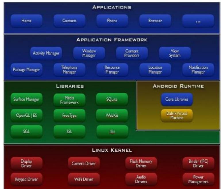
Fig. 1 Android System Architecture. Source: AISEC (2012)
