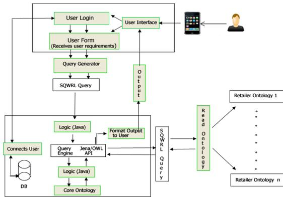
Figure 5: The Architecture of the Semantic Web Framework
