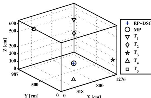
Fig. 8: Estimation positions based on Digital Sampling Oscilloscope measurements considering transmitters have different heights.
