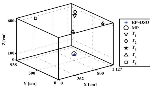
Fig. 6: Estimation positions based on Digital Sampling Oscilloscope measurements considering transmitters have the same height.
