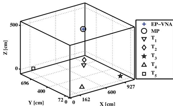
Fig. 9: Estimation positions based on Vector Network Analyzer measurements considering transmitters have the same height.
