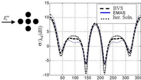
Figure. 8 the bistatic scattering cross section of five perfectly conducting cylinders each of radius =  $0.1\lambda$ , and their centers are separated by  $0.5\lambda$ , due to a plane wave incident at  $\theta_0 = 180^\circ$
