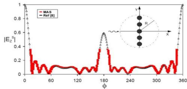
Figure.6 scattering by five identical conducting cylinders excited in x-direction with  $\rho = 5\lambda$
