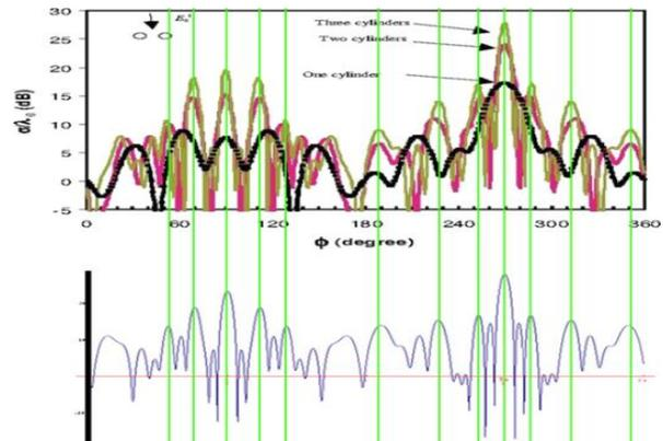
Figure. 12 The scattering cross section of three metamaterial cylinders located on x-axis with  $3\lambda_0$  center separation and a  $=1\lambda_0$  radius, metamaterial ( $\epsilon_r = -4, \mu_r = -1$ ). The angle of incidence is 90 degrees. The second figure shows the RCS according to MAS for three metamaterials
