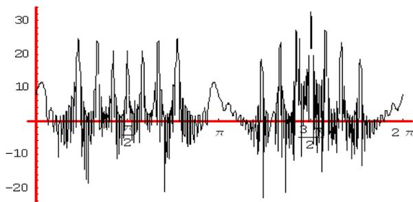
Figure. 9 RCS for 10 conducting cylinders obtained by global coupling.
