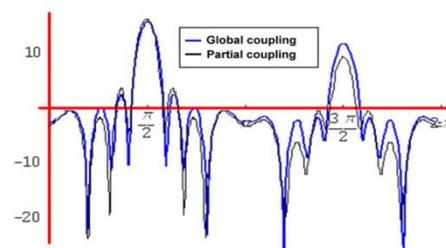
Figure. 7 RCS for five cylinders obtained by the global and partial coupling
