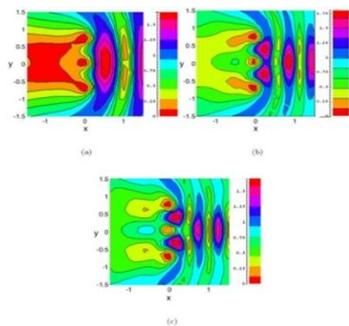
Figure. 4 Near field EMAS results for (a)  $\theta_i = 30^\circ$  et  $\varphi_i = 90^\circ$ , (b)  $\theta_i = 60^\circ$  et  $\varphi_i = 90^\circ$ , (c)  $\theta_i = 90^\circ$  et  $\varphi_i = 90^\circ$ .
