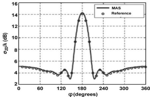
Figure. 2 The echo width results of a  $TM_z$  plane wave incident on a PEC cylinder of radius  $a = 1\lambda$ ,  $\theta_i = 45^\circ$ ,  $\varphi_i = 90^\circ$ .
