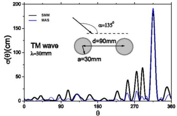
Figure. 11 Bistatic scattering width of two dielectric rods ( $\epsilon_r = 2 : 25$ ).
