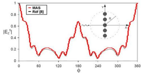
Figure. 5 Scattering by five identical conducting cylinders excited in x-direction with  $\rho = 3\lambda$
