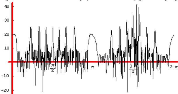
Figure. 10 RCS for 10 conducting cylinders obtained by partial coupling.
