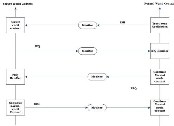
Fig. 6. Interrupt handling
