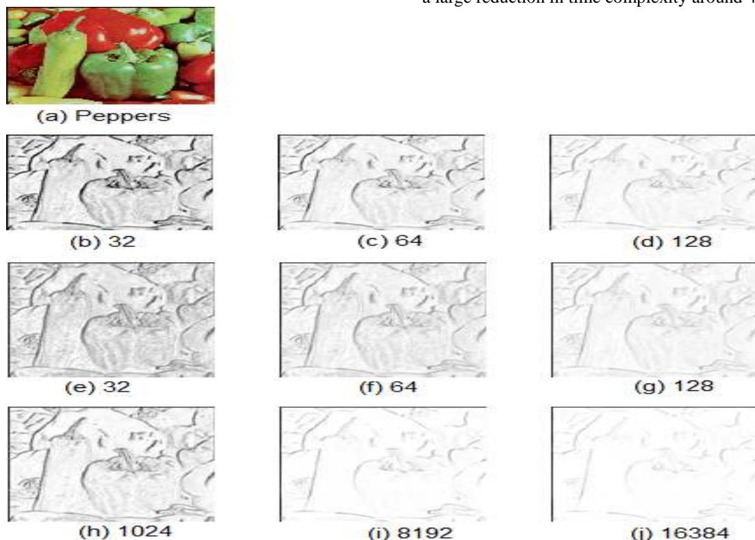
Fig. 4 Transformation of three-dimension color space into one dimension: Sa: (a) Peppers (b)–(d) By means of linear function with Dn: 32, 64 and 128. (e)–(g) By means of exponential function with Dn: 32, 64 and 128. (h)–(j) By means of Gaussian function with Dn: 1024,8192 and 16 384.
