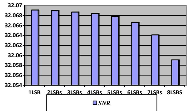
Figure 2: SNR vs. No. of Least Significant Bits
