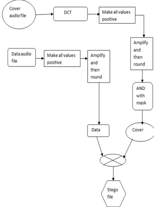
Figure.1: Block diagram of Audio Stegnography in DCT
