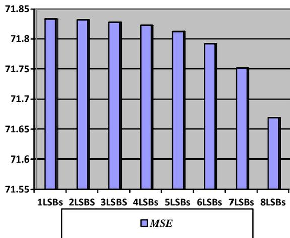
Figure 4: MSE vs. No. of Least Significant Bits
