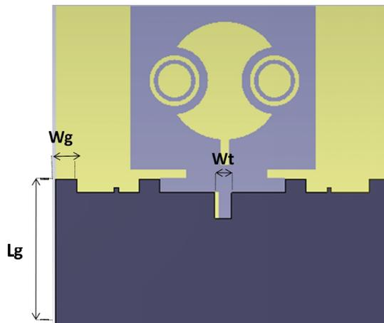
Fig 6: Slots in antenna and in ground plane.
