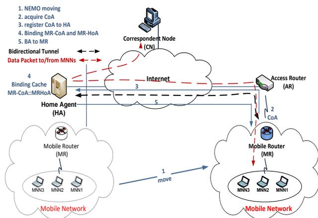
Fig. 1 NEMO BSP operation where numbers represent sequenced operation for NEMO
