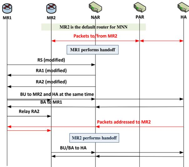
Fig. 5 Timing diagram for the proposed scheme
