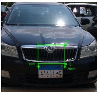
Figure 2: The relative position of Vehicle logo to the License plate
