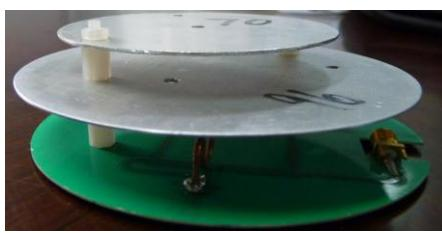
Fig. 6 Photograph of the fabricated antenna.
