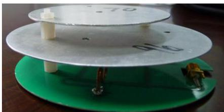
Fig. 6 Photograph of the fabricated antenna.
