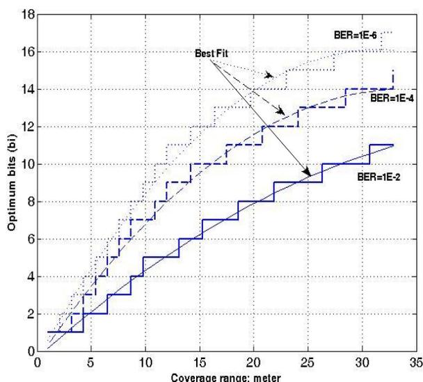
Figure (5): Optimum bit assignment with coverage range
