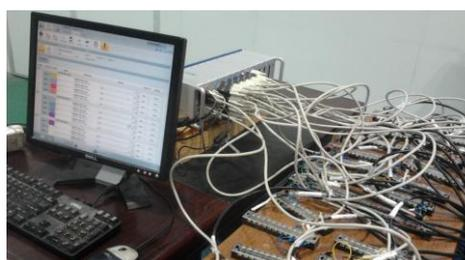
Fig. 9 24-channel multi-signal test System
