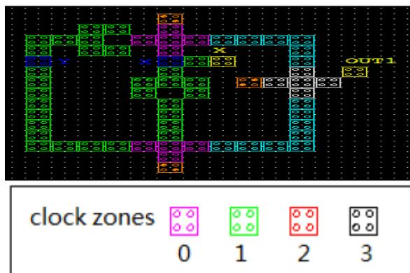
The Feynman gate layout has been simulated using QCA Designer version 2.0.3; a layout and simulation tool for QCA. The simulation results for a Feynman gate are shown in Figure 7.
