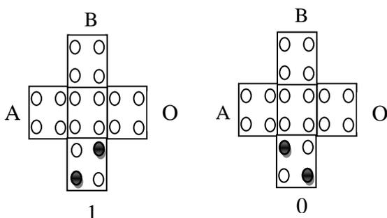
Fig. 3 2-input OR && 2-input AND gates.
