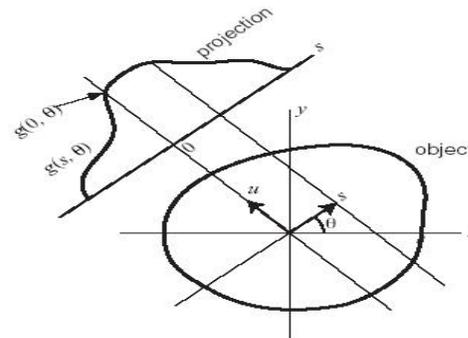
Fig 3. The Radon Transform computation.
