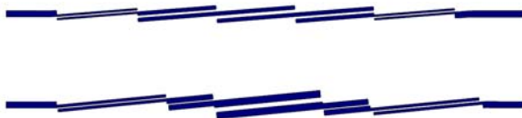
Fig. 6 Layout of (top) conventional BPF with \delta=0^\circ (bottom) modified BPF with \delta=30^\circ
