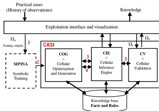
Fig. 3 General diagram of the cellular machine (CASI) [2]
